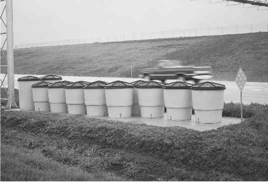
Figure 14-6. Example of sand-filled plastic barrels (the Energite III inertial barrier system) that protect vehicles from impacting bridge columns and other objects near highways. (Photo provided by Quixote Corporation, Chicago, IL.)
