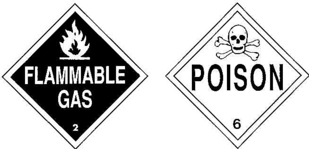
Figure 14-7. Examples of DOT warning placards.
