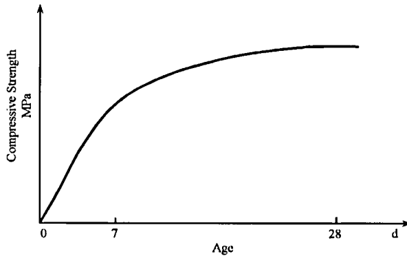
Figure 5.11 The Growth Curve of Concrete's Strength
