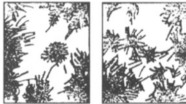
Figure 4.4 The Needle-like Crystals in Cement Paste
