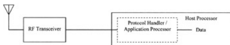
(b) Application processor and protocol handler integrated into host processor
