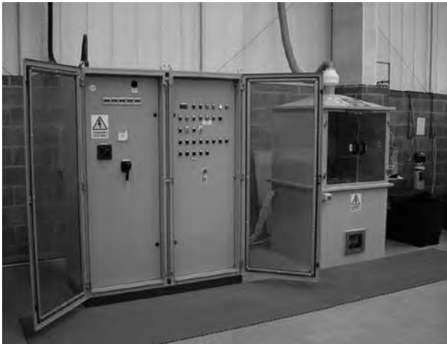
FIGURE 19.1 Keronite coating apparatus.
