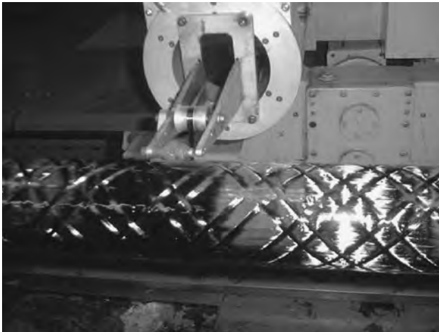
FIGURE 19.3A Filament winding of a CFRP prop-shaft.
