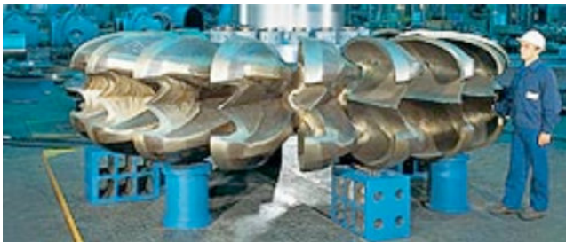
Figure 3.15 Photograph of a commercial Pelton wheel. Source: Voith Hydro.
