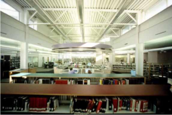
Figure 8.4 Daylighting example (NREL 09536).
