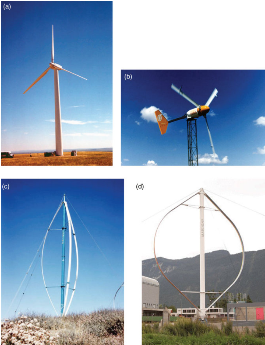
Figure 4.3 Examples of wind turbines. (a) HAWT (600 kW Mitsubishi); (b) HAWT (1.5 kW Bergey); (c) VAWT (FloWind Corporation 17 EHD); (d) Martigny wind turbine. Source: NREL.
