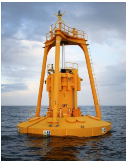
Figure 14.15 PowerBuoy point absorber above-surface portion. Source: http://images.nrel.gov/viewphoto.php?imageId=6471938 .
