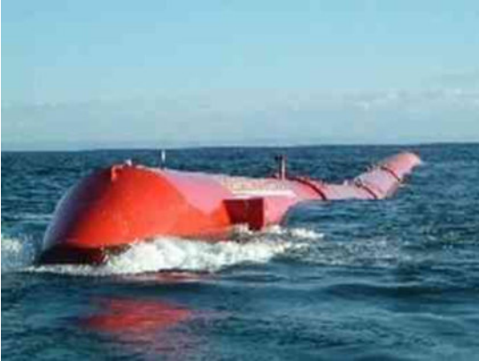
Figure 14.17 Pelamis P-750 articulated wave energy converter. Source: Pelamis.
