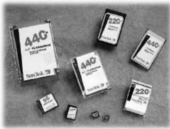
FIGURE 1.6 Illustration of Flash Memory
