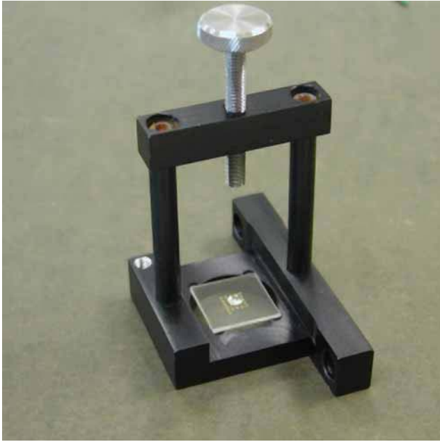
Fig. 3. Prepared array placed in the sample holder with the gold side facing down. The four corners cut into the holder are used as a guide. A drop of index-matching fluid is then placed onto the center of the glass side of the array.
