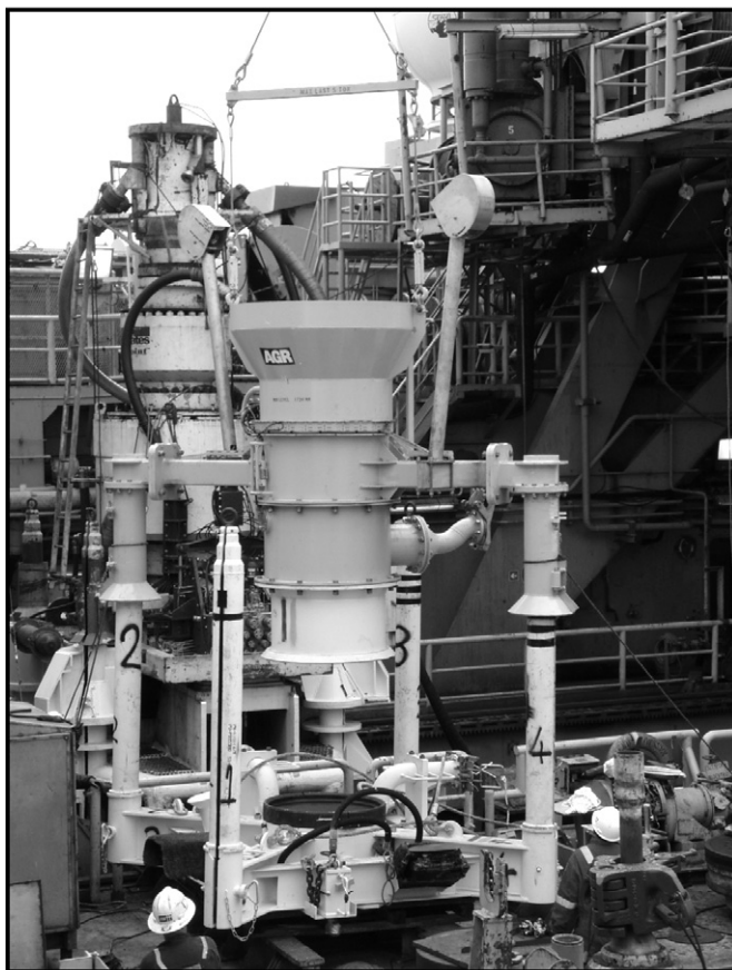
Figure 8.10 The wellhead component of the RMR system.
