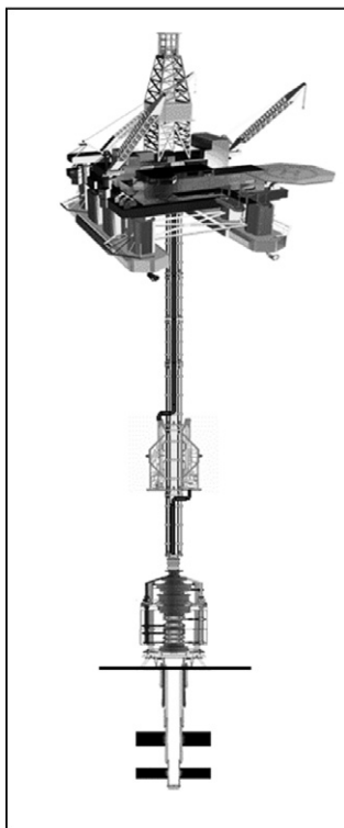
Figure 8.14 The pump deployed some distance above the BOP stack.
