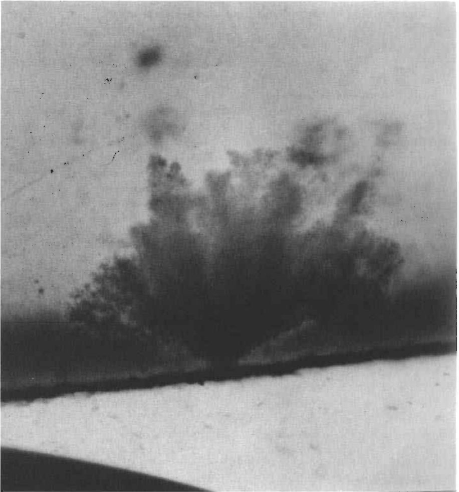
Fig. 9.3 Example of water treeing in a polymeric cable (courtesy of Dr J.C. Fothergill, University of Leicester)
