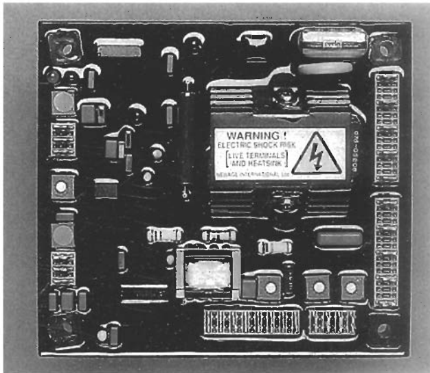
Fig. 5.12 Layout of an automatic voltage regulator (AVR) (courtesy of Newage International)
