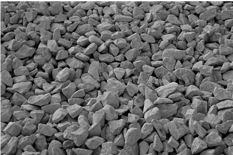
Figure 5.3 A coarse-aggregate sub-base provides good structural support and drains well, but is hard to grade precisely
