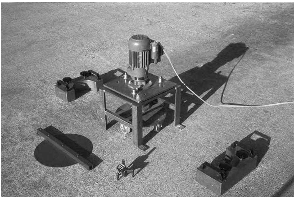
Figure 20.2 Chaplin abrasion tester
