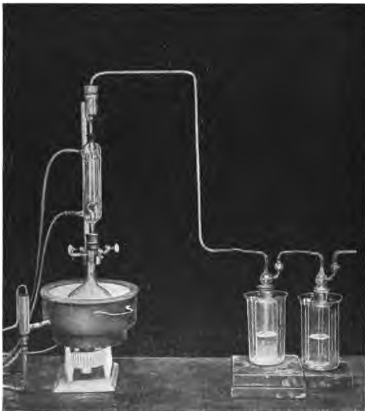
Fig. 95. Preparation of acetaldehyde. Distillation of the aldehyde and absorption in ether.
