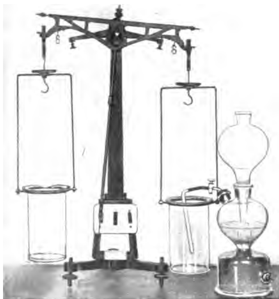
Fig. 32. To show that carbon dioxide is heavier than air by weighing on a sensitive chemical balance.
