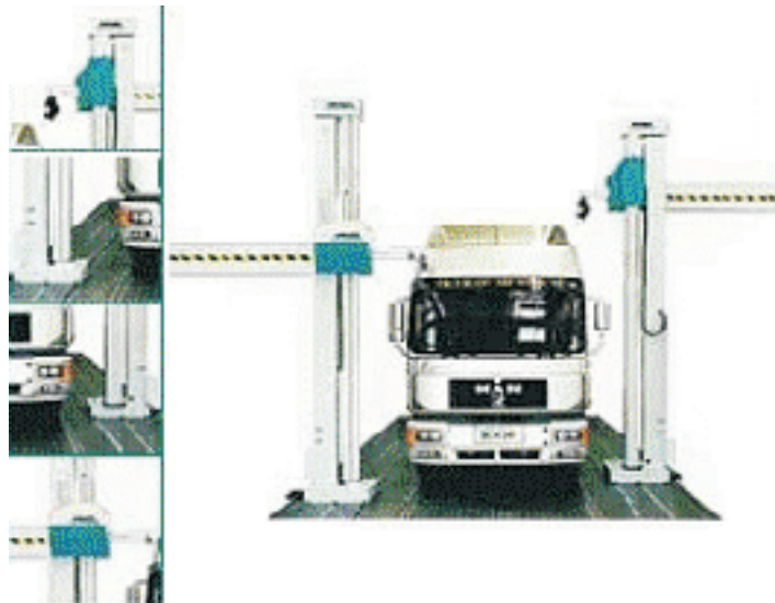
Fig. 7.3 Horizontal CMM on inspection work
