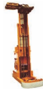
Fig. 8.5 Side loading and high lifting type
