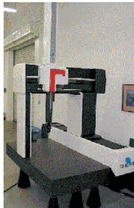
Fig. 7.9 DCC (Direct Computer Control) CMM
