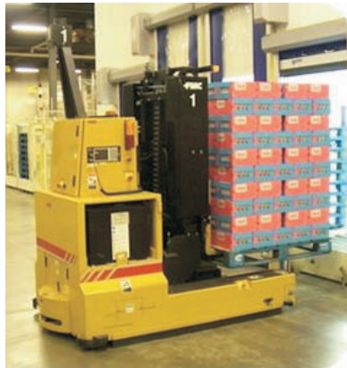
(a) AGV in plastics industry handle raw materials and finished
