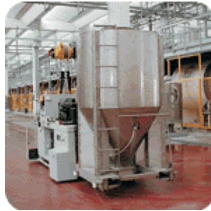
(b) AGV in chemical industry to handle raw materials are goods finished goods
