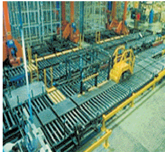
Fig. 8.20 ASRS Crane—High-rise storage of work in process, including weighing and profiling of loads before storage
