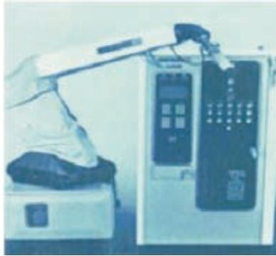
Fig. 8.30 Robot performing spray painting
