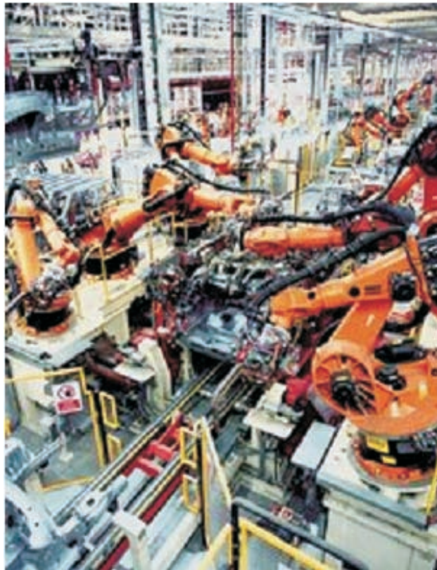
Fig. 8.35 Industrial robots doing vehicle underbody assembly (courtesy: KUKA).
