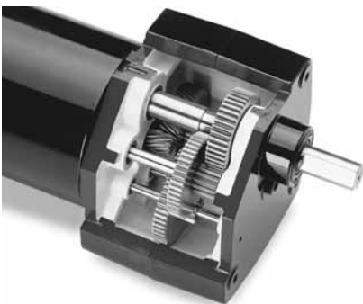
Combination of spur and helical gears can be seen in this cutaway view of a sub-fractional horsepower parallel-shaft gearbox. Note multiple gear stages.
