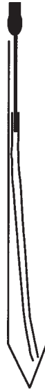
Fig. 2. Hypodermic needle with a piece of polyethylene tubing attached in a 15-mL plastic tube.
